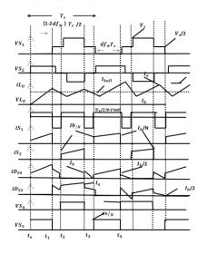
Fig. 6. Waveforms in the charging/forwarding mode
